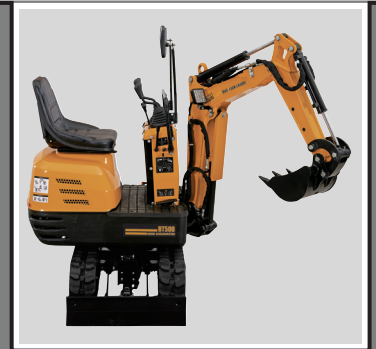
Easy switch from boom swing to upper structure swing.
