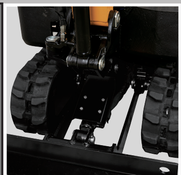
Shielded hydraulic cylinder
